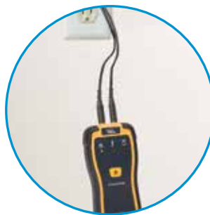
Traces on de-energized circuits
